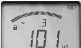
The display shows "3" for the third measurement for the specific label. The arrow sign to the left only represents the omitted characters to the left of the digit "3".
