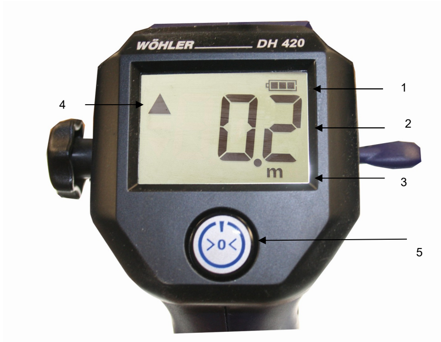
Fig. 9: Display and control button
