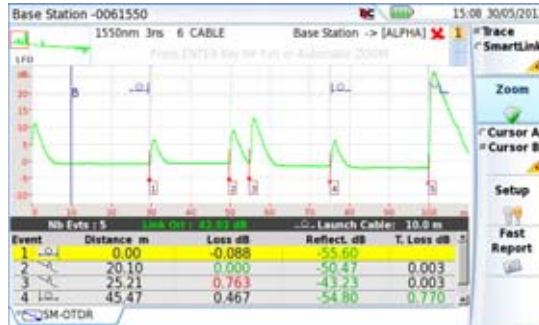
Figure 71 FTTA OTDR Trace
