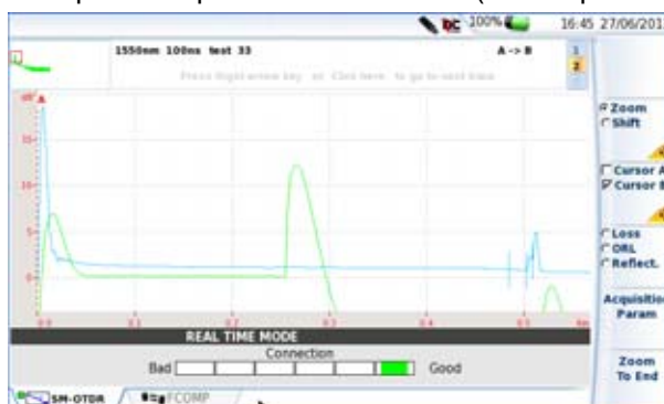
Figure 23 Example of acquisition in Real Time (with Expert OTDR)
