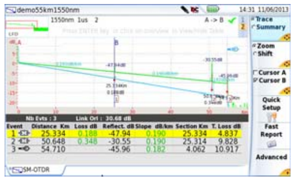
Figure 32 Example of trace and results table in Expert OTDR
