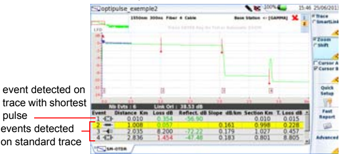
Figure 52 OTDR Traces with OptiPulses
